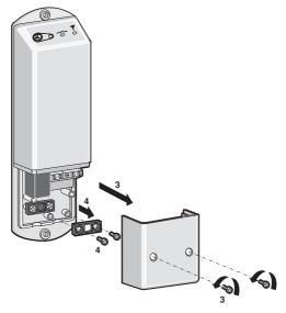
4 Unscrew both screws of the lower right cable bracket and remove the bracket.
